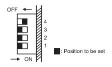
**NOTE:** Make sure that bits 1 to 3 of the Piano key switch are set to OFF. These bits are used for inspection at the factory. If you use the In-Skin Router with bits 1 to 3 being set to ON, we cannot guarantee its proper operation.
